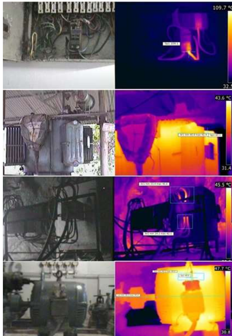
Fig. 7: Visual and its respective thermal images of different electrical and mechanical systems.
