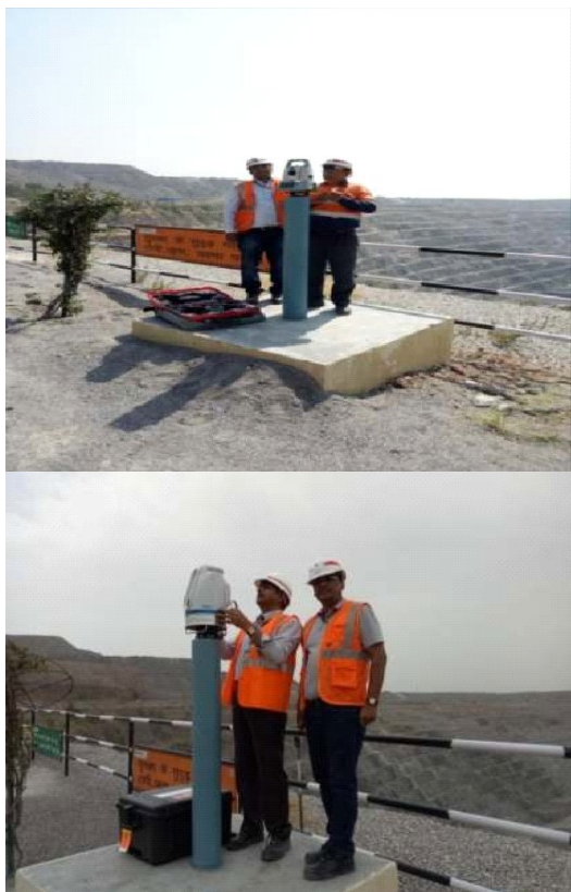
Fig. 7: Monitoring observations with Total Station & 3D Terrestrial Laser Scanner
